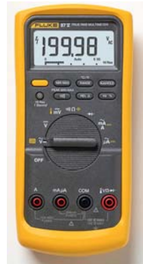
Figure 7.6. The Fluke 87V can measure temperature.
